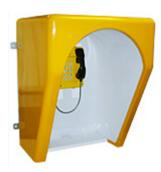
For external or internal use, the T5000 Marine is designed to attain a high level of noise reduction up to 23dB. Manufactured using general-purpose resin mat to BS476 Class 1 fire retardancy, the T5000 Marine is extremely robust and weatherproof. Inside the hood's outer shell is a perforated polypropylene lining that houses 50mm non-hygroscopic acoustic insulation.
